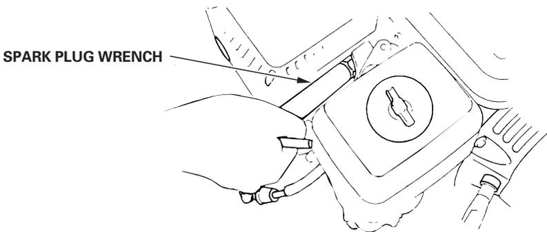
3. Visually inspect the spark plug. Replace the spark plug if there is apparent wear, or if the insulator is cracked or chipped. Clean the spark plug with a wire brush if it is to be reused.
