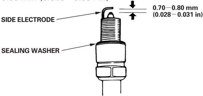
5. Check that the sealing washer is in good condition, and thread the spark plug in by hand to prevent cross-threading.
