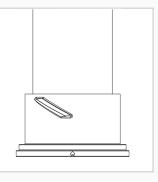
4] Completely remove the Bin to gain access to the Liner.
