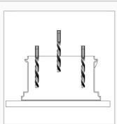
3] Using Fixing Plate as a guide, drill 3 x M10 holes 80mm deep.
