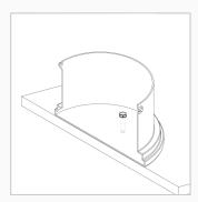
4] Secure the bin to the base using 3 bolts. Place liner into bin to cover over fixing.
