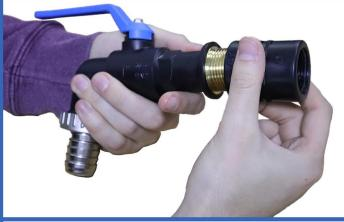
4. Thread the 1" female coupling onto the 1" BSP bib tap.
