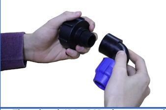
1. Thread each IBC x BSP adaptor to each MDPE elbow adaptor.
