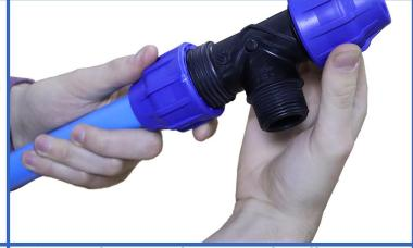
3. Insert the pipes between the elbows and tee pieces. Twist the collars to tighten.
