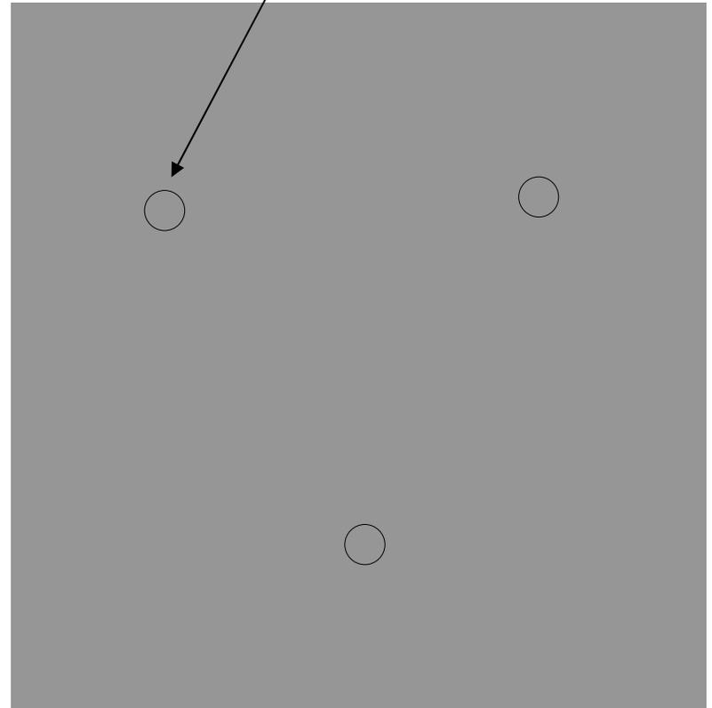
Using a 16mm masonry drill bit drill the three marked holes and insert the ground anchor sleeve
