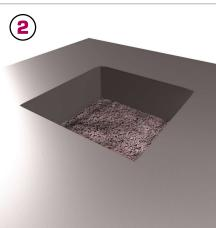
Dig a hole of size 550 x 550 x 260mm deep. Fill with 50mm compacted hardcore as
