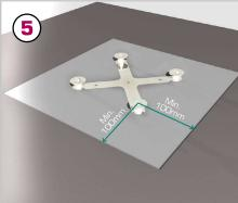
Once level and correctly positioned, pour concrete in carefully in order not to displace fixing. Once filled, recheck the placement and adjust accordingly.
