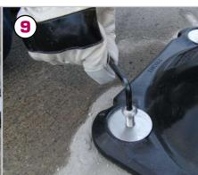
The fixing screws should drop down until they sure all four bolts are engaged in the shield thread by 2 or three turns then proceed to tighten all four bolts to torque setting 27.
