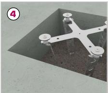
Insert the Concrete Ground Anchor keeping a minimum 100mm distance to any edge of the hole. The spacer plate should be flush with the ground level.
