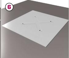
When the concrete has set remove bolts, washer, spacers and spacer plate.
