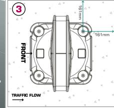
Survey the installation site to ascertain suitability for the product and location. Check for buried services and prepare site if necessary, be of size 550 x550 x 210mm deep.
