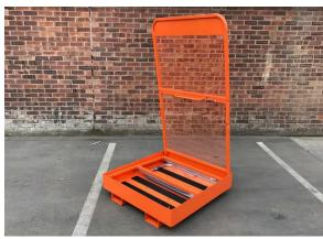
**Step 3** – Lift the front section guard through 90 degrees and lock the fixed pin into the vertical slot. The Guard will be locked in position and leaning forward slightly.
