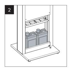
Sit the containers into the base. Remove the lids and peel back the safety cap.
