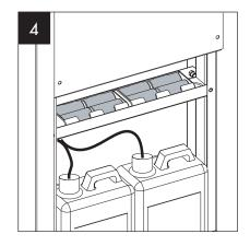
Insert the provided batteries into the battery holder. Take care to ensure all batteries are inserted with the correct polarity as shown inside the battery compartment.
