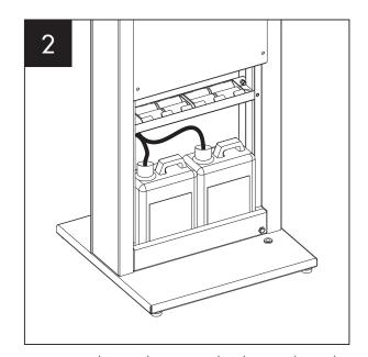
Remove silicone hoses and either replace the sanitiser containers or top up as required. Insert the hoses back into the bottom of the containers.
