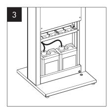
Insert the hoses into the containers ensuring they are pushed to the bottom.
