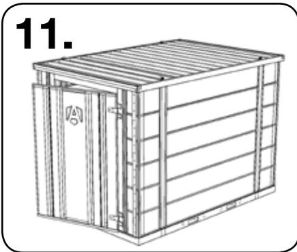
Now place the roof on top. An extra person may be needed inside the unit to balance the roof.
