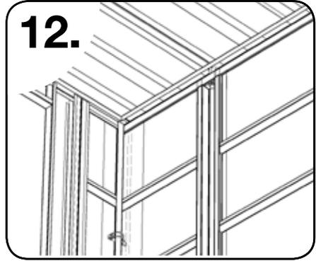
Ensure the grooves in the roof fits in the top of the 4 panels all the way around.
