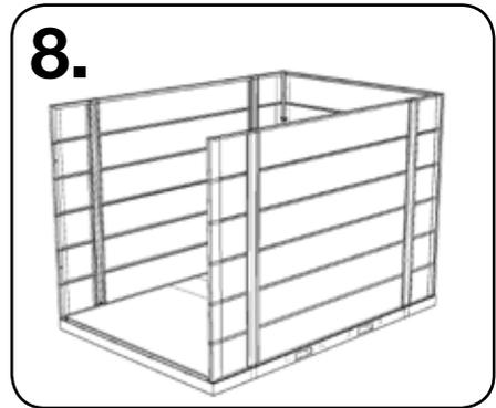
Place the other side panel on the base, and secure it with bolts as described in step 3.
