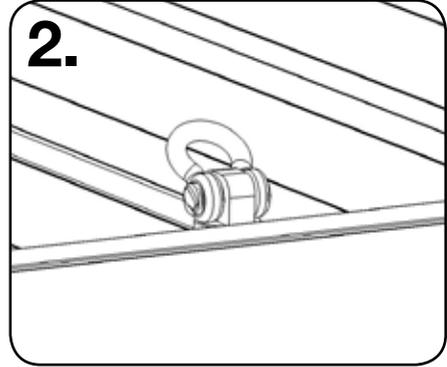
Attach the lifting equipment to all four lifting eyes and ensure that the load is lifted evenly across all four eyes.
