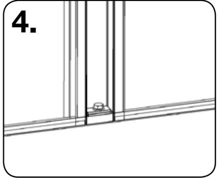
Ensure it is supported safely while the 45mm bolts are fixed in, securing the side to the base.
