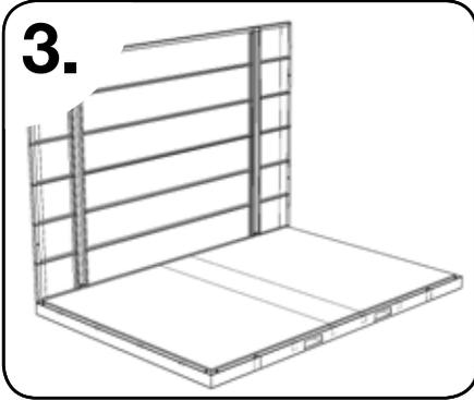
Place one of the side panels on the base, using the bolts in step 2 to locate the panel.
