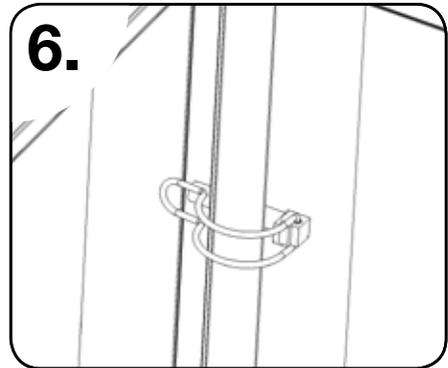
Put a pipe linchpin through the rear panel and side panel to hold them together.
