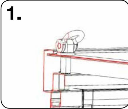
Before lifting, ensure that the bolts holding the lifting eyes are securely in place.
