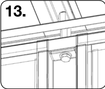
Lastly, fix the roof in place using the bolts provided.
