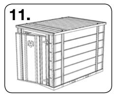
Now place the roof on top. An extra person may be needed inside the unit to balance the roof.
