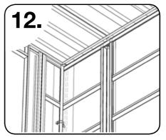
Ensure the grooves in the roof fits in the top of the 4 panels all the way around.
