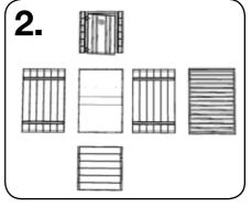
The roof is removed first, followed by the door panel, a side panel, the rear panel and the remaining side panel. Fixings can be screwed back into the panel afterward for safekeeping.
