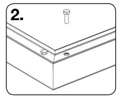
Bolt in the 20mm bolts into each corner of the base, two to every corner.
