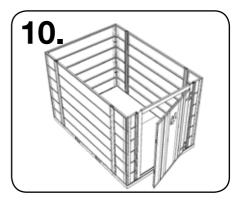
The door panel is the last panel to be fixed on. This slots onto the base and is fixed to the side panels with linchpins as described in step 5.
