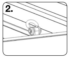
Attach the lifting equipment to all four lifting eyes and ensure that the load is lifted evenly across all four eyes.
