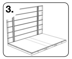
Place one of the side panels on the base, using the bolts in step 2 to locate the panel.
