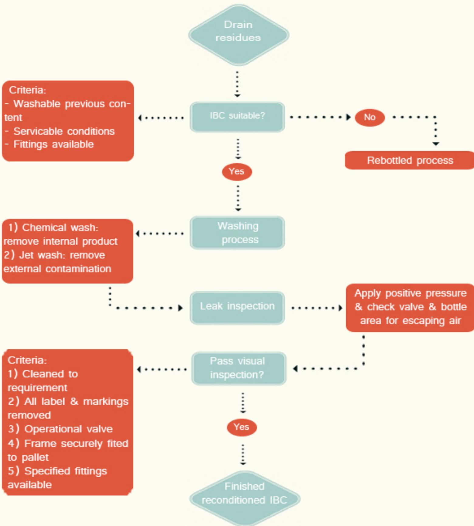
Although these IBCs have been professionally cleaned, they could have previously contained any type of liquid or chemicals and traces of this liquid could still remain in the bottle.
