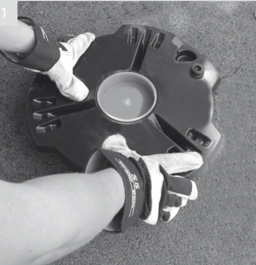
Position the ballast cartridge so that the locking pin is at 45° in a clockwise direction from the direction that the lock on the bin will face
