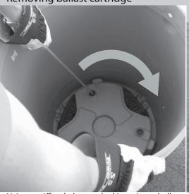
Using a stiff rod, depress locking pin on ballast cartridge, whilst pushing down twist bin body anti-clockwise, rotate until bin is free
