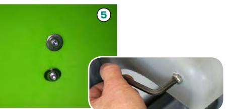
With both eye mouldings in position fully tighten up the dome head bolts using a 5mm allen key.
