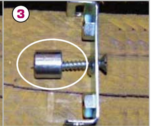
Place the metal spacer tube over the end of the screw as shown.
