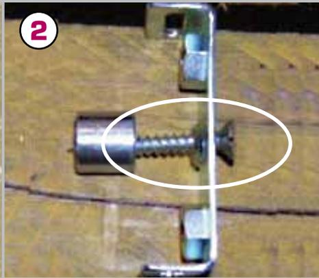
Insert wood screw through the centre hole of the 'U' bracket.
