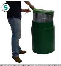
Place steel liner back inside of plastic body.
