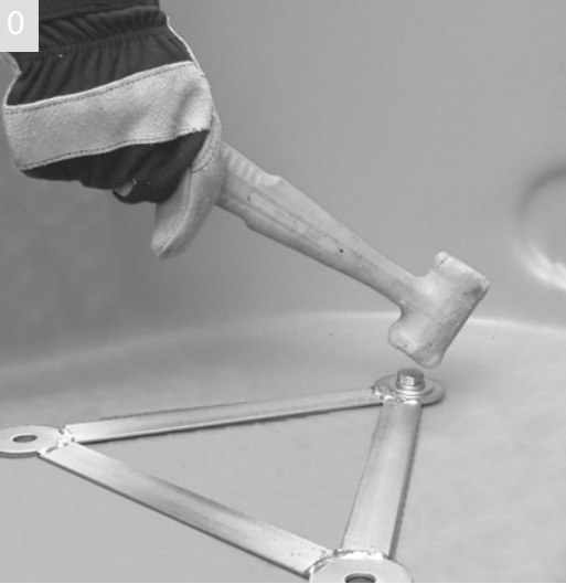
Put washers onto bolts. Push bolts into the three holes and drive them home with a hammer
