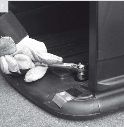
7 Use a spanner or socket to tighten the bolts
