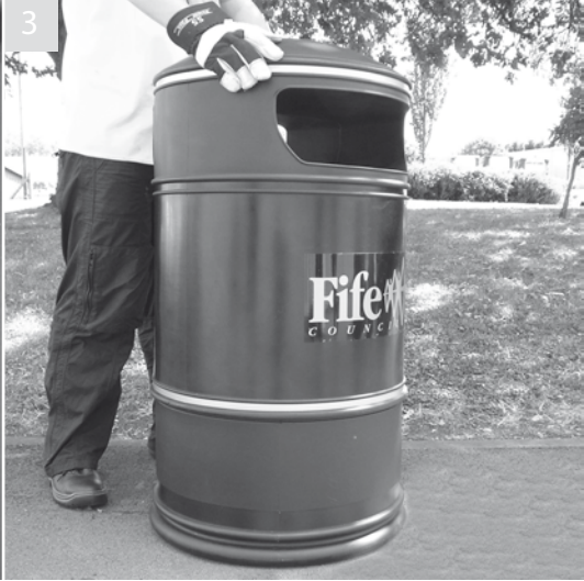
Replace liner and hood. With hood resting on base rotate hood clockwise until it will rotate no further. Push lock in to engage
