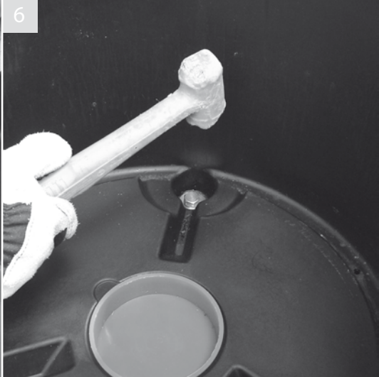
Using a mallet drive the bolts home
