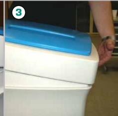
With one hand at the back of the bin push the lid towards the back and lift away.
