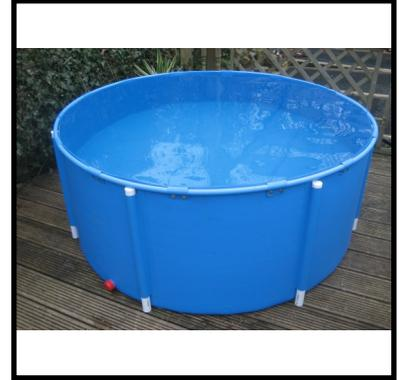
These high quality temporary koi carp vats are manufactured in the UK using high grade, 1mm thick PVC coated polyester joined using specialised RF plastic welding techniques to give leak free welded seams.
