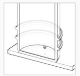
4] Secure the Bin to the Base using 3 bolts. Place liner into bin to cover over fixing.
