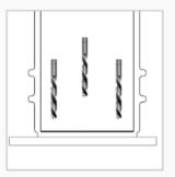
3] Using Fixing Plate as a guide, drill 3 x M10 holes 80mm deep.
